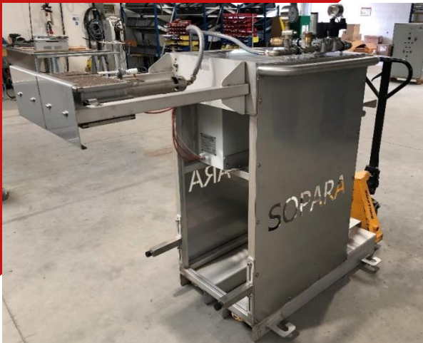
Mobile trolley allowing the rapid installation of the radiant between the tools
